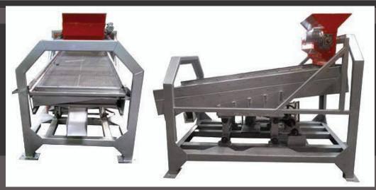
The Quail II eccentric cleaner is used for the removal of most foreign material from the raw product being screened, based on size. The eccentric cleaner removes all particles that are larger or smaller than the raw material being cleaner, including particles such as metal, dust, stones, husk, and sand from the grain. The screening may be followed by an aspiration process whereby all light particles are removed through an air channel.
