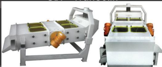
The Francolin vibration cleaner is a grader and is used for the removal of most foreign material from the raw product being screened, based on size. The vibration cleaner removes all particles that are larger or smaller than the raw material being cleaner, including particles such as metal, dust, stones, husk, and sand from the grain. The screening may be followed by an aspiration process whereby all light particles are removed through an air channel.
