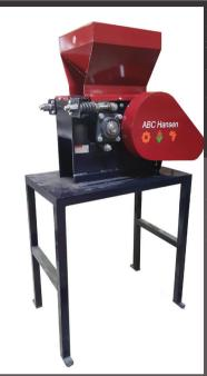
The ABC Hansen maize crusher is a simple roller crusher for breaking maize kernels and pellets, using 2 x 250mmØ x 200mm wide rollers – one driven and one free running
