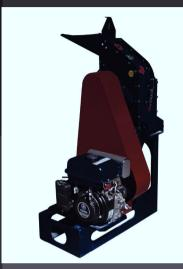
The design of the Baby HIPPO HAMMER MILL is unique in that there are no chopping knives, as the material is being fed directly onto the tips of the rotating hammers in the direction in which the hammers are rotating. The milled material is gravity fed out the front of the mill at a convenient bag off height of 850mm. A wide range of screens is available, from 25mm down to 0.6mm aperture
